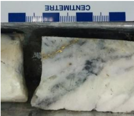
Figure 26. Core photo of coarse free gold in the high-grade Swann Zone (Fosterville Deposit, 2017, M.S. King site visit).
